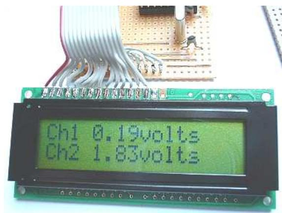
Figura 2.7: Display LCD 16X2
