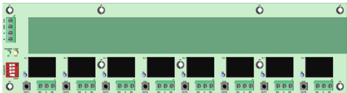
Figura 2.47 Interfaz CCO (Contact Closure Output)
