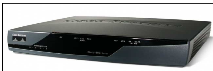
Figura 2.1 Router Cisco 851 Series.
