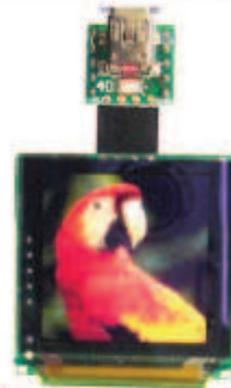
figure 3: Interface to any 4D serial device such as the uLCD-OLED and uVGA modules with the extra 5pin header provided.
