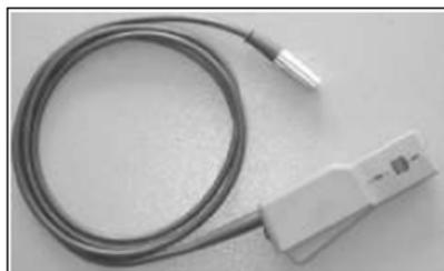
**Figura 4-15:** Pinza trigger.
