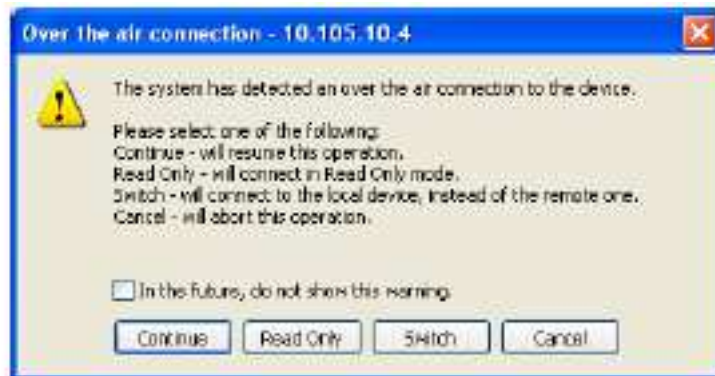
Figure 2-9. Over the Air Connection
