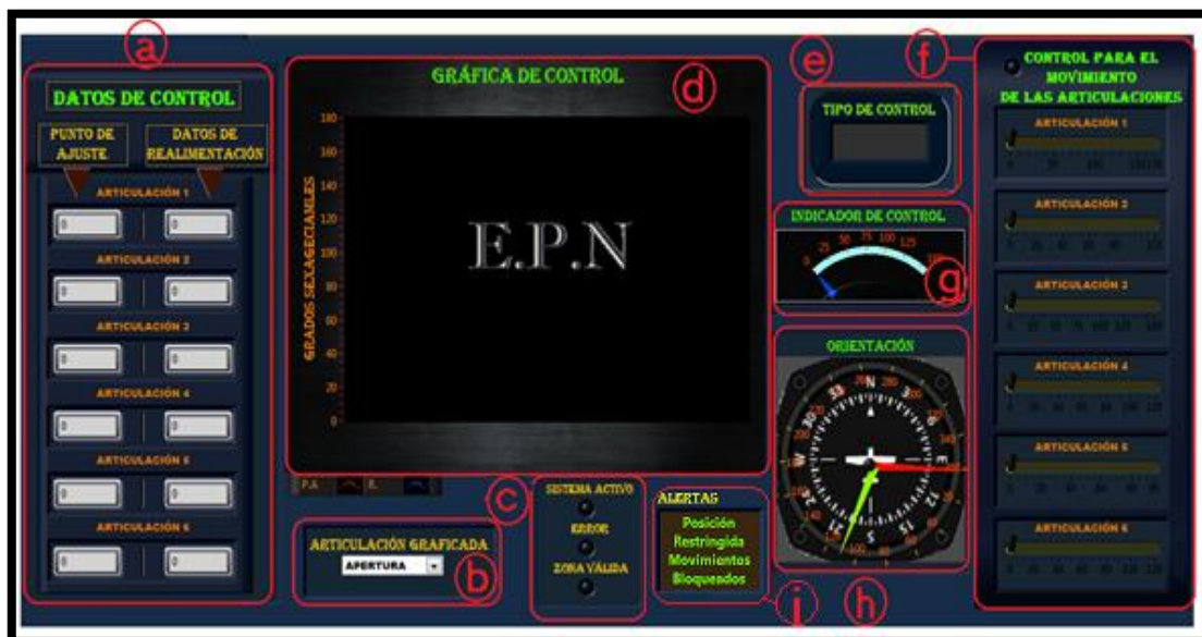
Figura 3.33 Panel de control del HMI
