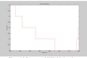
Figure 15. Response of V/Hz Limiter (frecuency)
