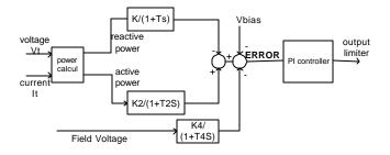
Figure 11. Simplified Model of Underexcitation limiter [6]
