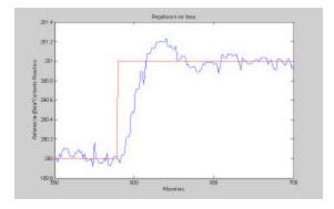
Figure 6. Response of Automatic Voltage Regulator from a machine connected to the power grid
