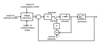
Figure 3. Block Diagram of Automatic Control Voltage and Manual Control
