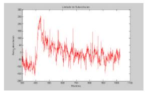
Figure 13. Response of Underexcitation limiter (error signal)
