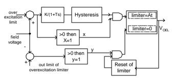
Figure 7. Model of Overexcitation limiter
