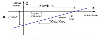
Figure 10. Straight line limiting characteristic of an underexcitation limiter [6]
