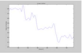
Figure 16. Response of V/Hz Limiter (Terminal Voltage)
