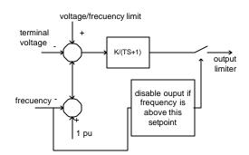
Figure 14. Simplified Model of the V/Hz Limiter
