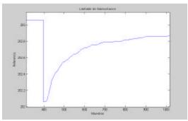
Figure 12. Response of Underexcitation limiter (Voltage reference)
