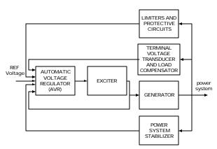
Figure 1. Functional block diagram of a synchronous generator excitation control system [2]
