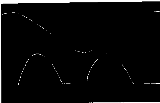
Figura 16 - I_{aEF} = 24 \text{ A} ; V_{eEF} = 80 \text{ V} ; \alpha = 93,27^\circ
